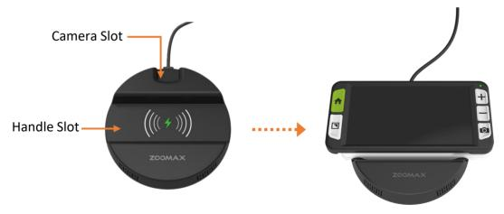
Wired Charging: Connect the adapter directly to the Luna 6 via the USB-C port on the top edge of Luna 6.
