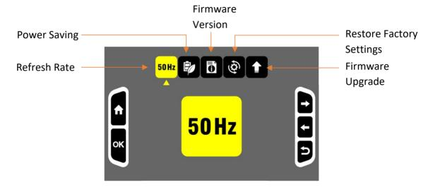
To select an option in the System Settings, move the Zoom in/out button to cycle through the icons, and press the Mode button to confirm. Press the Freeze button to go back, or the Home button to exit.
